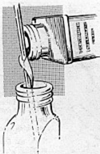
To fill small-mouthed bottles pour liquids down a rod held in contact with mouth of bottle. Paul M. Trach, Prince Albert, Saskatchewan.
