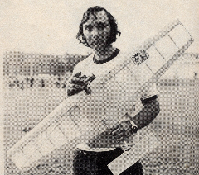
Gene Pape looks unhappy, but his airplane is the best around. A built-up copy of Rich Brasher's foam Rotation Station, it needs extra spars on the left wing to prevent roll instability.
