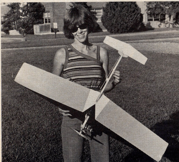
Rush's modification of Gary James' foamy has long tail for maneuvering stability and forward sweep for upwind performance. Joanne Bartley is the better-looking model, however.
