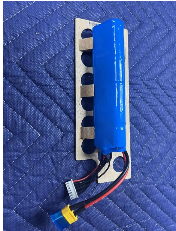
Li-Ion battery on new battery plate
