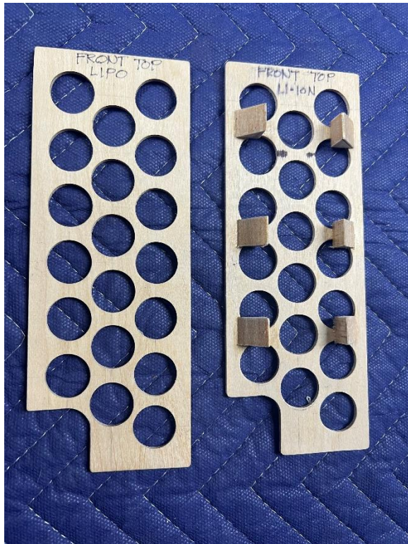
Li-Po battery plate (left) and Li-Ion plate (right)
