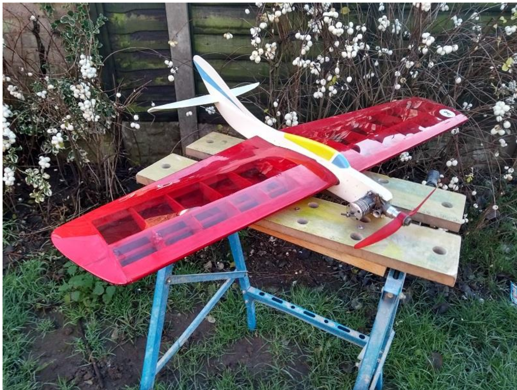
Peacemaker, for 2.5-.19 motors 35 1/2" span. Built by me
