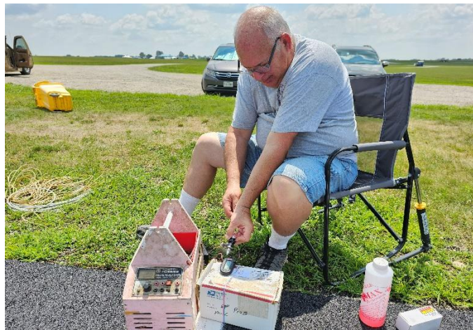
Mike Greb from Texas shows brave form as he holds his running Cox .049 by his bare his fingers in front of his tachometer.
