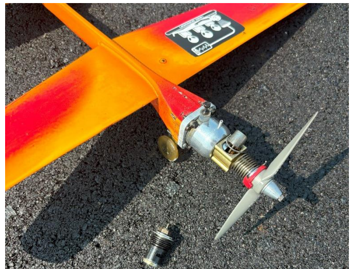
Doug's Mouse 1 entry showing sheared crankcase threads.
