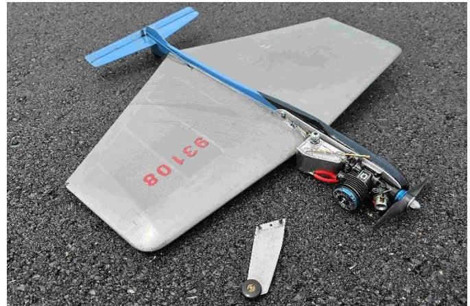
Bob Oge's pilot cleaned off his LG on his slow rat due to a control failure.
