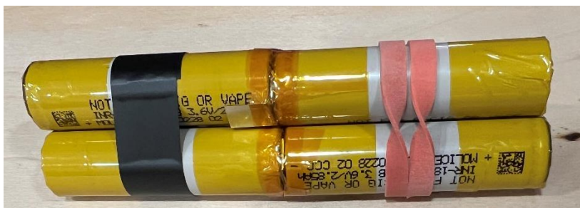
Adding Electrical Tape to Hold the Banks Together
