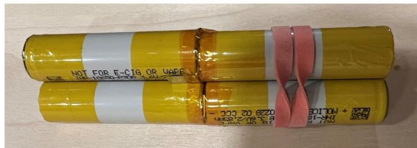
Use a Rubber Band to Temporarily Hold Banks Together
