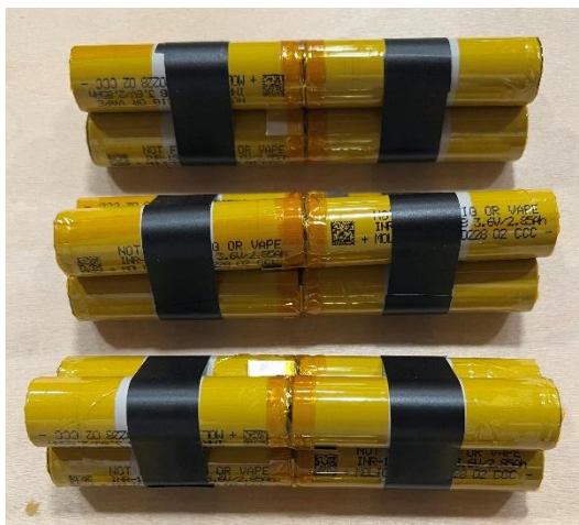
Battery Pack Held Together with Electrical Tape
