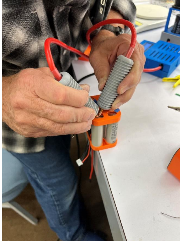
Jimby spot welding a 5-cell Brick-Type Battery Pack (Notice the Orange End Caps)
