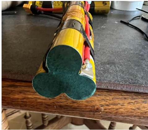
Fish Tape on End of Battery Pack
