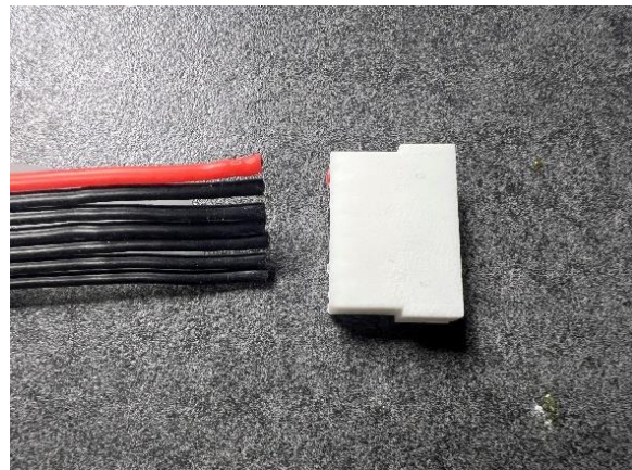
Cut Off the Male Connector of the 6S JST-XH Balance Plug Extension Lead
