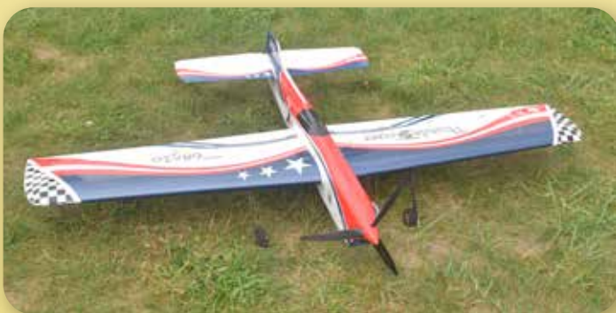
Dave Fitzgerald USA had a Thundergazer III powered by a PA-75. It is painted with dope and automotive clear.
