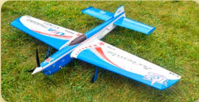
Matthew Colan USA flew his own design Artemis. It is a balsa construction with a weight of 1,9 kg and powered by a PA-75. Paint scheme from the World Baseball Classic Team USA. Randolph dope and automotive clear.
