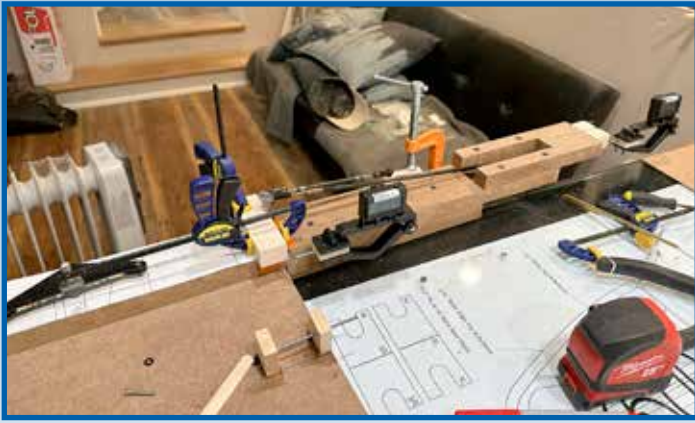
"Ironbird" jig for controls fabrication.
