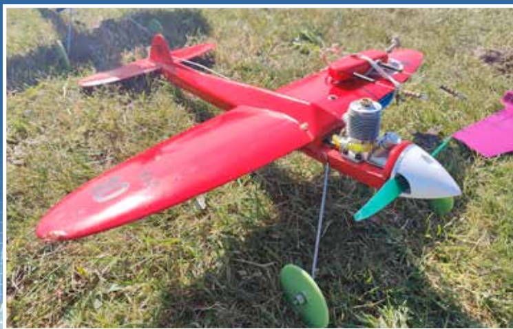
Jörgen Aagaards model with a Parra Wasp 1,5 cc diesel
