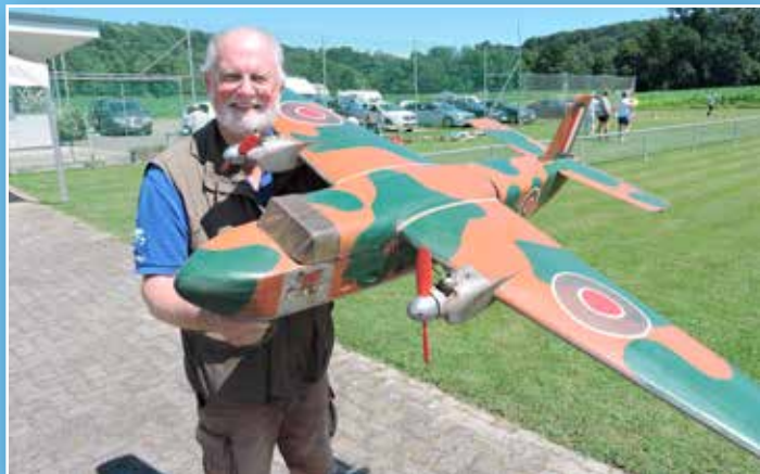
The author and co-organizer Heimo Stadlbauer with a twin-engine transport machine from the 1950s, powered by Webra Mach I 2.5 cm 3 Diesel engines.
