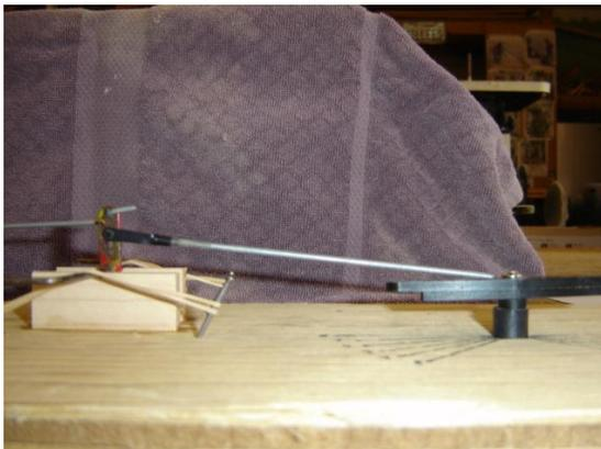
I then set the elevator end of the flap to elevator pushrod to the closest hole to the control horn rotation axis. The Ted Fancher article gives measurements and refers to these positions as fast or slow. The closer the hole location to the rotational axis of the particular control, the "slower" (or less) the control movement outcome. Conversely, the further the pushrod hole from that rotational axis, the "faster" (or more) the control movement outcome.
