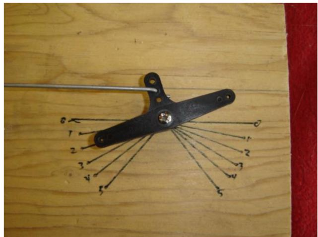
In the first observation, I set the bellcrank to flap control horn pushrod to the second hole in from the furthest end of the bellcrank and to the second hole down from the “top” of the flap control horn
