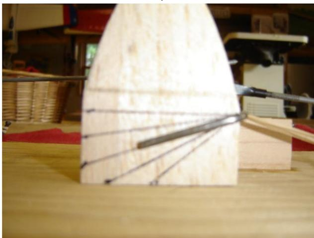
10 degree Flap 11 and Elevator 17 20 degree Flap 20 and Elevator 30 30 degree Flap 33 and Elevator 50.
