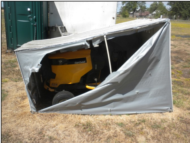
Sunlight aged the south tarp (installed 2017)
