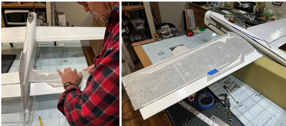
Applying the Paint Masks to the Stabilizer and Wing
