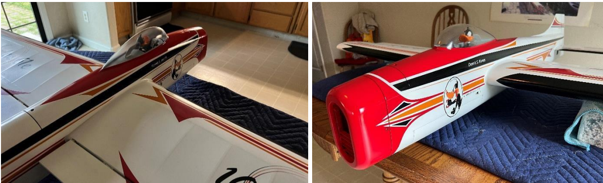
Circulas 61e after the first coat of clear prior to sanding
