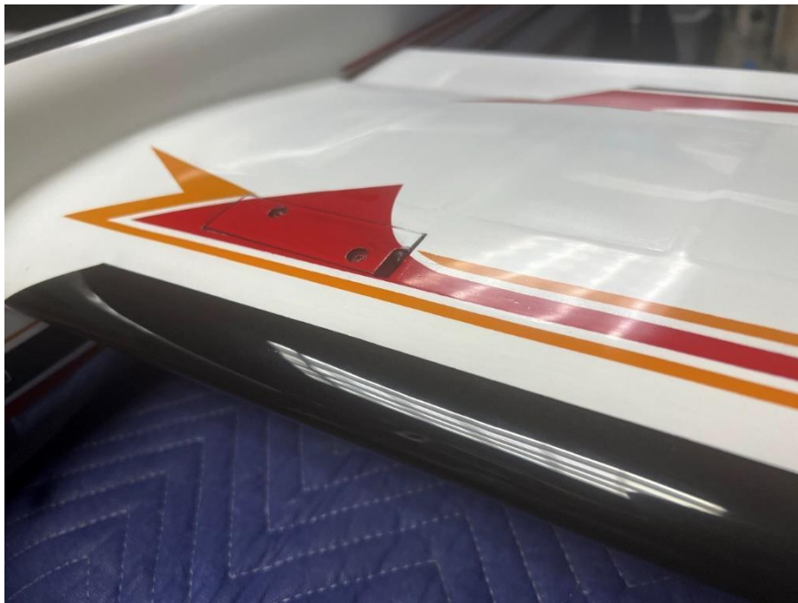
Circulas 61e after sanding and polishing the clear coat
