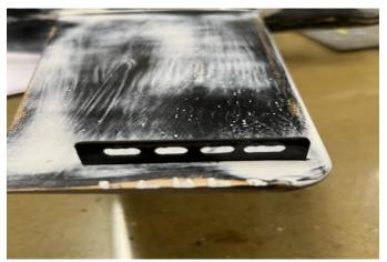
My adjustable wingtip was cut from a sheet of carbon & then bonded into the wing.
