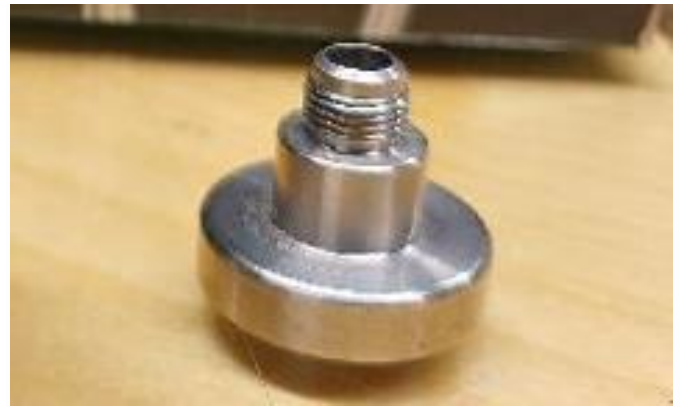
What the fixture looks like. Fits most engines that use Nelson taper seat plugs.
