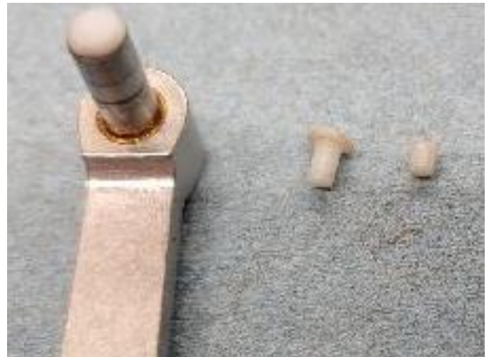
Shown is the broken pad, the remade pad and the installation of the new pad in the wristpin. * Note how the edges are rounded on top.
