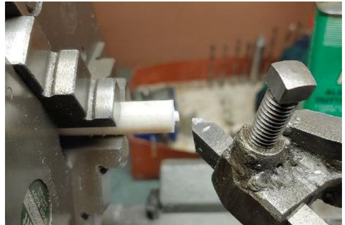
Start with piece of Teflon rod & a sharp tool bit. First cut on the Teflon rod is to the outside dimension.
