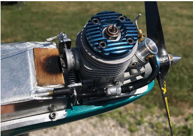
The “Flippy” end of Tim Stone’s Slow Rat, GO .25 for power. Note the “scorched” plywood heat shield glued to the fuel tank to prevent erratic runs.
