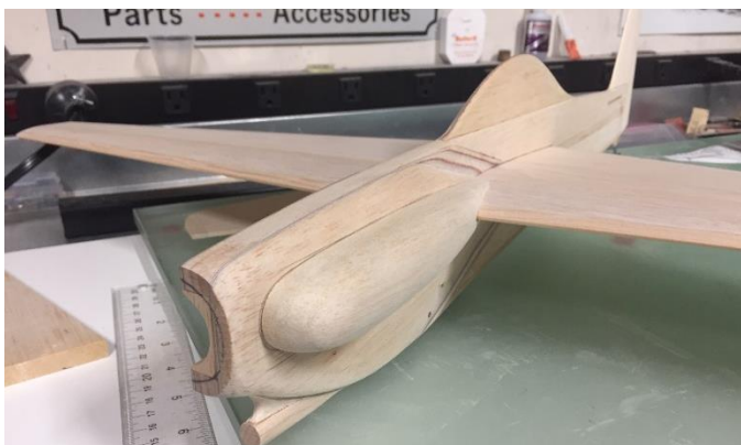
Kelly Hite's Invictus, built from Doug Mayer's plans. Will have SH 15 power.
