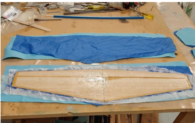
Layup before going into the vacuum bag.
