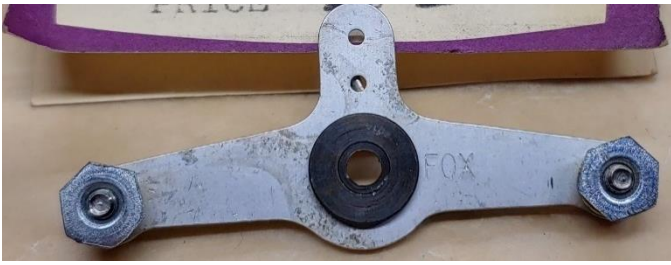
Part of Bill's hardware package included this Fox Bellcrank with line Buttons added.
