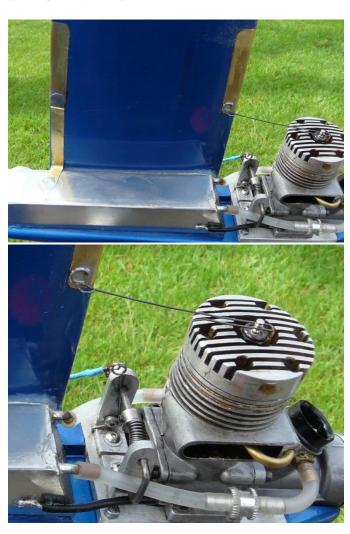
On a Quickie Rat, the preferred location for the contact points is on the leading and trailing edge of the wing as shown. The leading edge contact connects directly to the glow plug post, and the trailing edge contact connects to the engine crankcase, using the fuel tank as part of the circuit.
