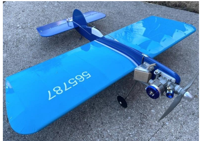
Kelly Hite's new Clown Racer. Externally modified O.S. 18 T.Z. for power, See Column for details.
