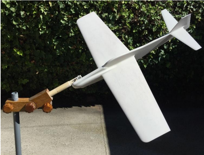
Look at the fancy jig Dave Hull made for holding his '74 Shoestring model during painting.
