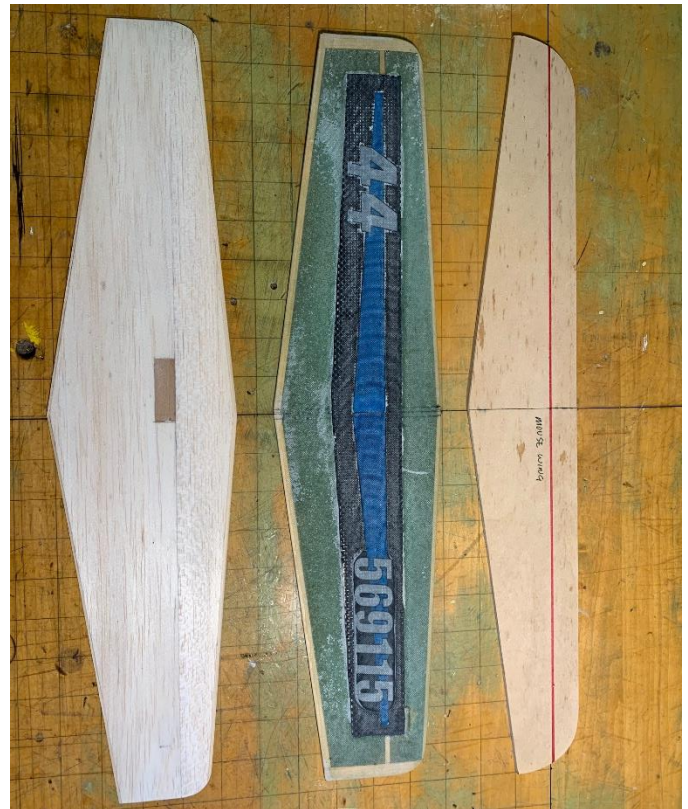
I took this photo of one of my Mouse Wings, the Divinylcel wing, and the new balsa wing for comparison.
