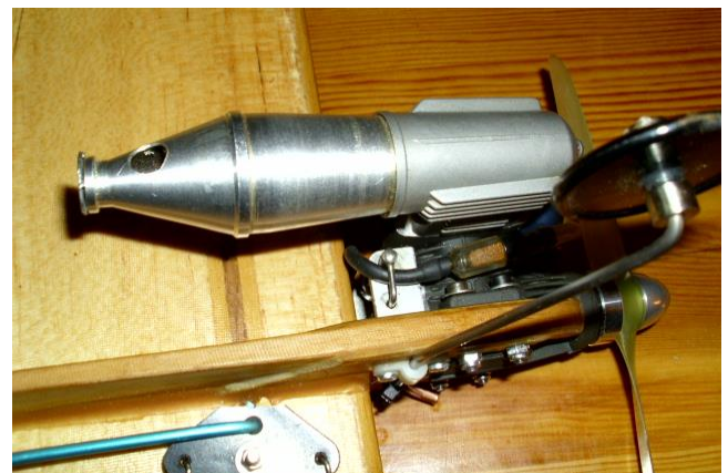
Engine: "FORCE .21 CNC" + OS/F2D Combat muffler and prop @ RTF Combat lines (0,38mm /0.015).
