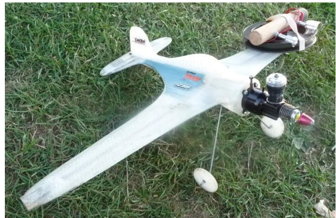
And finally, a fully printed " Hummel " mouse racer from Sebastien Kunzke of Germany and it flies well!
