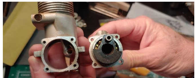
Can you tell me what's wrong here in this photo? Yes, the front crankcase gasket is missing!
