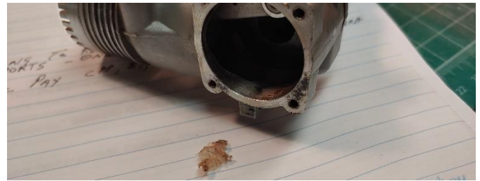
Indeed the wrapping paper the seller used somehow found its way inside the motor!
