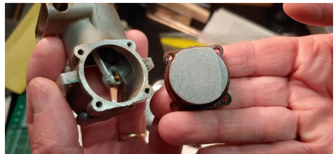
This is how the back plate should look with its proper gasket in place.
