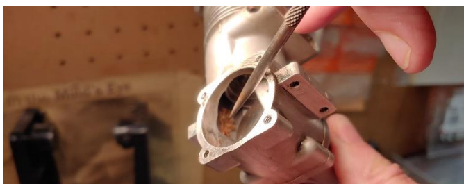
Note that I found what appears to be the packing material lodged up in the bypass port!
