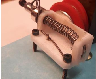
Tony Toogood from the U.K. makes these fabulous racing wheels as well as a fuel shutoff with a 3D printed frame. See text for details.
