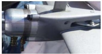
Note venturi air hole in fuselage just ahead of the bellcrank slot.
