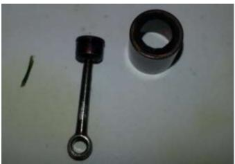
Above: This is what happens when one neglects the resetting of the ball-socket joint of a Cox .049. Ingested grass is bad too.
