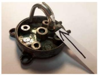
Incorrect fuel attach tubing allows for leakage at the backplate nipple as well as where it attaches to the aluminum pick up tube.
