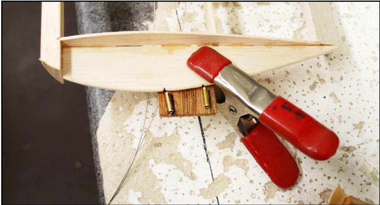
A guide for drilling 3/32" holes through a 1/8" wingtip. Gene Pape photo.
