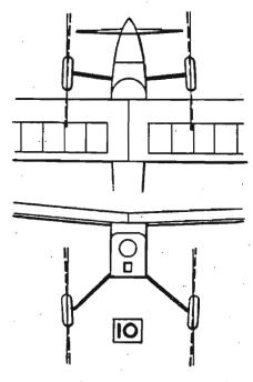
alignment (10). From the top view slight "toe-in" can be tolerated and from the front a little "camber" if desired in order to prevent the wheels splaying out.
