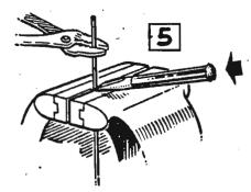
With one end of the wire held firmly in the vise jaws, the other can be bent by hand with a few licks of a hammer near the bend (3). Have a paper gear pattern nearby (4) and check the accuracy of the part by superimposing it from time to time. Small corrections in the angles can sometimes be made with
