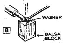
a soft balsa block after the inner washer is slipped onto it (8). The block positions the washer and holds it perpendicular during soldering. If acid-core solder is used, carefully wipe all traces of the
