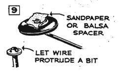
acid away with a cloth; coat with oil. See that the wheels fit the axles snugly but freely, bush them with thin wall tubing if necessary, then slip on the wheels. With a piece of thin balsa or sandpaper as a spacer between the outside of the wheel hub and the washer, solder the washer in place (9).
