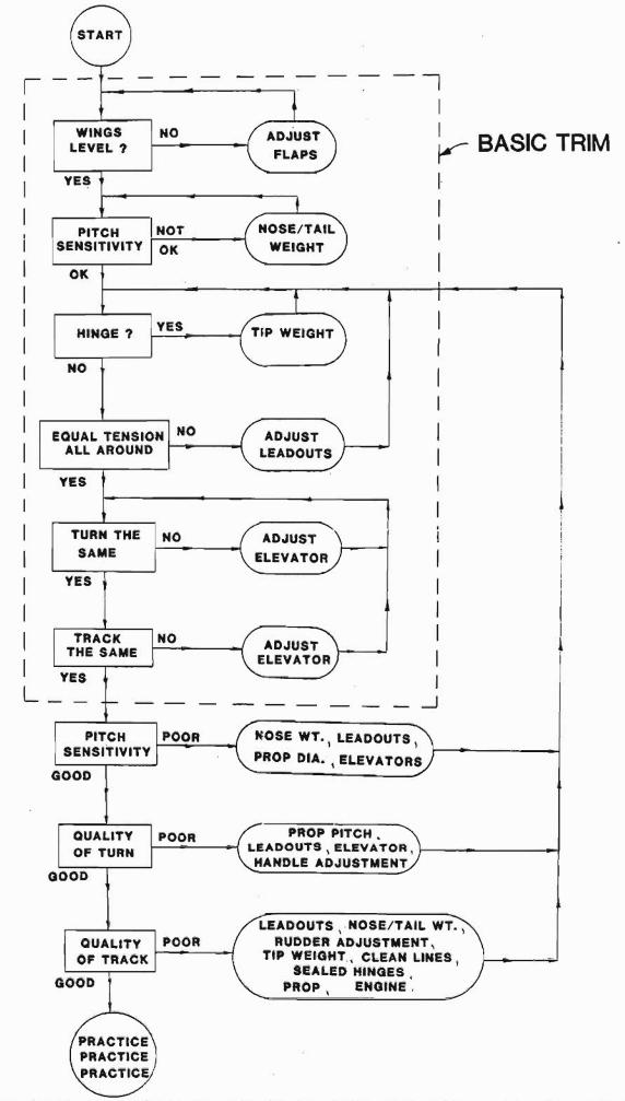
what you have just done to get it to turn the same. If this is the case, make it track the same and adjust the turn now with an adjustable handle. This completes the more objective part of trimming and now comes the more subjective part, which makes all planes fly different. This trimming can take a lot of flying to be happy with. This stage is very personal
