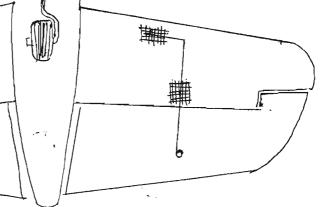
No, it wont interfere with the control of the plane when you need to give some "down"; I didn't say to use 3/16th" wire! I've used it on my CORSAIR for three years.
