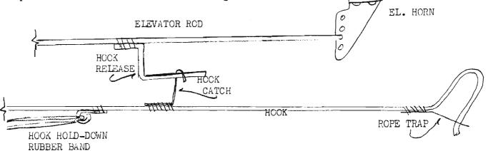
Above, you see the Z-shaped hook release wired and soldered to the elevator rod. You also see the hook catch, made of finer wire, .026". The rope trap and hold-down were covered in an earlier article.
