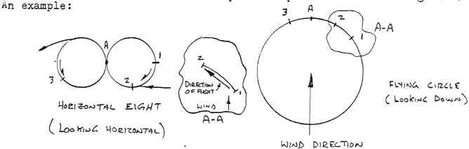
A horizontal eight. Entry (Point A) is directly down wind. At point 1, the plane is pointed directly down at the ground. But, between 1 and 2, the wind now has a component in the same direction as the direction of travel. This will increase the speed of the plane. This is most noticable from point 1 to 2 as the plane is also being worked upon by gravity, tending to increase
