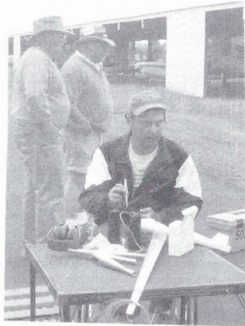
Ron Salo works on his speed ship at the NW Regionals. The asymmetrical bird is .15 powered and has monoline control system. (Beers photo)
