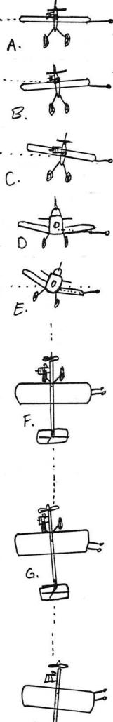
If you looked carefully, you saw that the model hung so that it was slightly rolled inboard, toward the pilot, if it were in a flying attitude. Now do you recall all the times you have been flying a RINGMASTER and found yourself looking at the top of the inboard wing? Thought it was a wing warp, didn't you? Fellow hooker, it was ...
