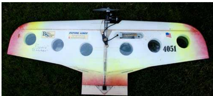
Plane is Jeff Dawson Sonic Chicken. Power is Fora .36. Prop APC 7.8x6.
