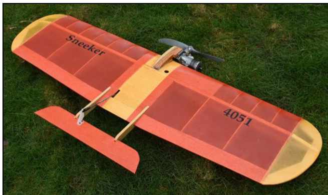
John Thompson's new Sneeker, built from a kit made by Gene Pape, powered by Johnson .35. Finish is Plyspan and clear dope.
