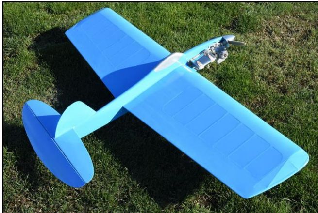
Mike Hazel's Ringmaster 576, a Pat Johnston design, power by O.S. .46 LA. Finish is Monokote and epoxy.
