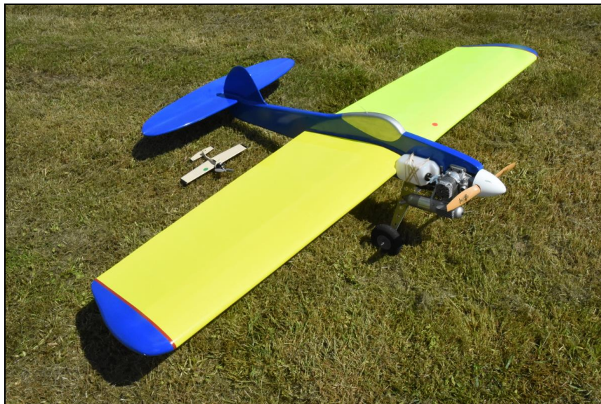
Mike Hazel's big Ringmaster, 73 inch wingspan, powered by O.S. .90. For comparison, his Micro Ringmaster, powered by Cox .010.
