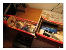
Upgraded to Solid State ESC and LiPol battery pack. that it cut the weight to 4 1/2 pounds. It flew, but still short of power. Brushless motor next.
