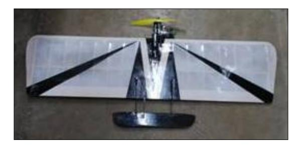
The clear material was given a mist coat of Rustoleum white primer before I ironed it on. No other adhesive was required. The material can be trimmed with dope, however this model is trimmed with black Econokote. If you check out the sources below, you will see that you can have a lifetime supply of this material for less than \$50.00.
